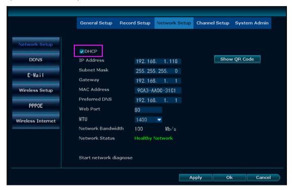
2 If still show offline, please have a check at the Ethernet cable and see if the Ethernet cable has the problems. Try to use the Ethernet cable for other device and see if it works.
